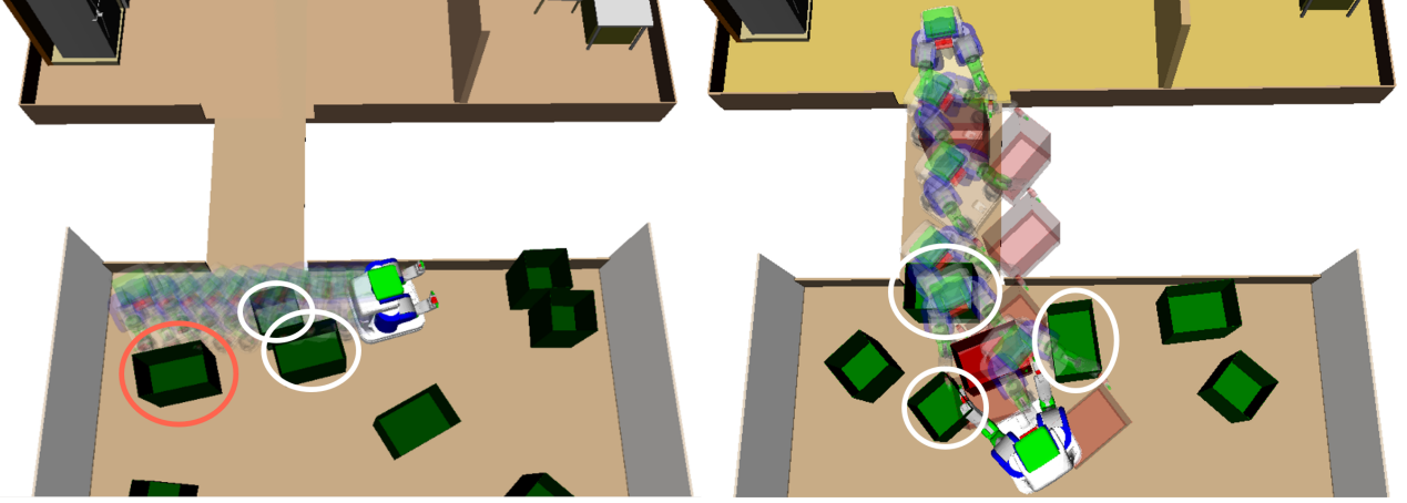
Figure 5. Example evaluations of OCCLUDESPRE (left) and OCCLUDESMANIP (right). In the left figure, the robot is trying to pick up the box marked with the red circle, and plans a motion whose swept-volume is shown with the transparent robots. There are two obstacles, marked with white circles, in collision with this motion, making \text{OCCLUDESPRE}(o_{\text{white}_1}, o_{\text{red}}) and \text{OCCLUDESPRE}(o_{\text{white}_2}, o_{\text{red}}) to true, and \text{OCCLUDESPRE}(o, o_{\text{red}}) to false for all the other movable objects o \in \mathbf{O}^{(M)} . In the right figure, the robot is trying to move the red box to the kitchen region located on the top, and plans the manipulation motion whose swept-volume is shown with the transparent robots. There are three objects, marked with white circles, in collision with this motion, so \text{OCCLUDESMANIP}(o_{\text{white}_i}, o_{\text{red}}, r_{\text{kitchen}}) is true for i \in \{1, 2, 3\} , and \text{OCCLUDESMANIP}(o, o_{\text{red}}, r_{\text{kitchen}}) is false for all the other movable objects o \in \mathbf{O}^{(M)} .
